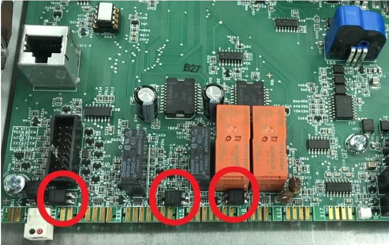
Figure 2. New-Style shunts
